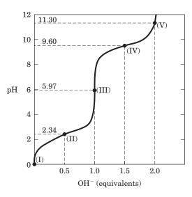
**3.** How Much Alanine Is Present as the Completely Uncharged Species? At a pH equal to the isoelectric point of alanine, the *net* charge on alanine is zero. Two structures can be drawn that have a net charge of zero, but the predominant form of alanine at its pI is zwitterionic.
