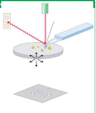
FIGURE 1 The principle of atomic force microscopy.
